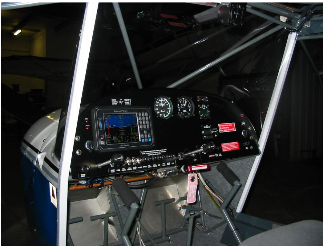
Optional glass panel with backup Airspeed and Altimeter and radio and transponder shown
